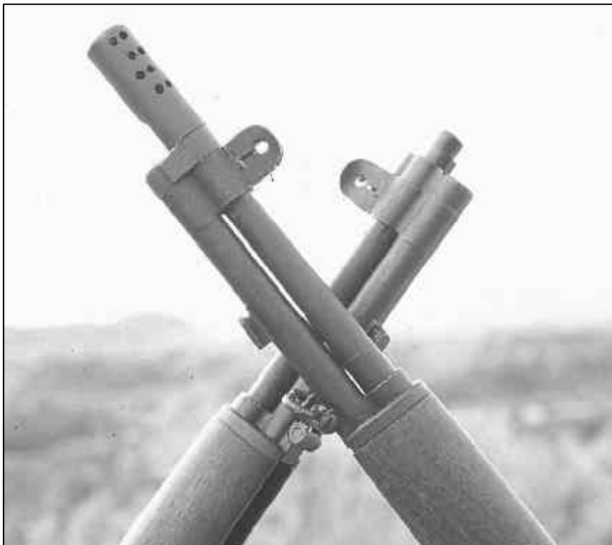
Left: With the gas cylinder and barrel of a standard Garand in the background, the “Type E” Garand retained the M1 gas cylinder, but added a muzzle brake to better control fully automatic fire.
