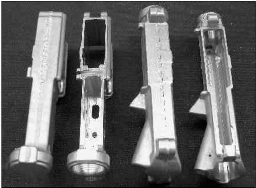
Above & Below: Initial forgings of Bushmaster upper and lower receiver assemblies on the left with their machined counterparts to the right. After machining is done they still must pass another stage of inspection before being finished with a baked dry-lube film and Hard Anodized with a Nickel Acetate final seal coat.
