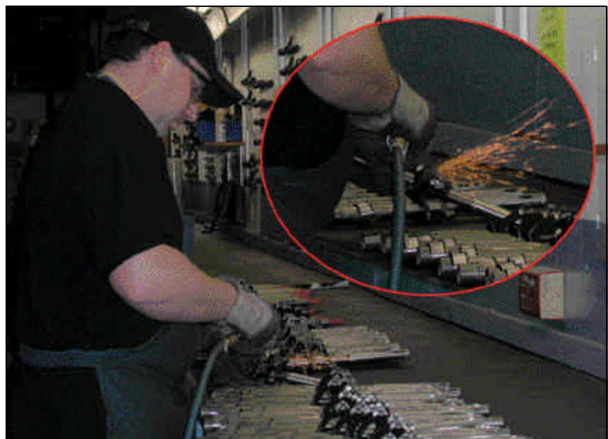
Below, Right: Sights are checked for uniformity and “adjusted.”
