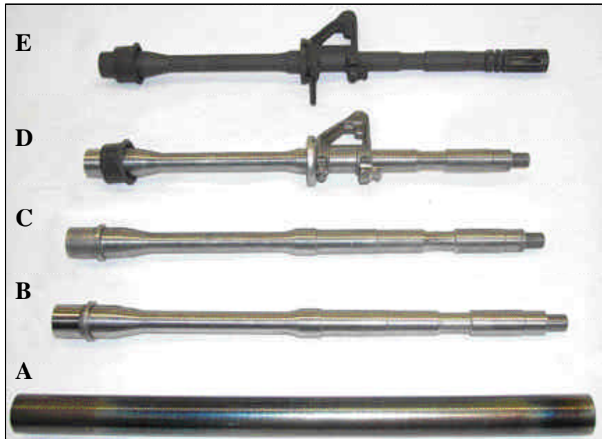
Above: The barrel manufacturing process involves several steps. A) The stock material is drilled, button rifled and stress relieved. B) It is then turned and head spaced. C) The barrel is next chrome lined. D) The gas port is drilled and the front sight is indexed. E) After passing several quality control checks between each stage, the barrel is finally phosphate finished.
