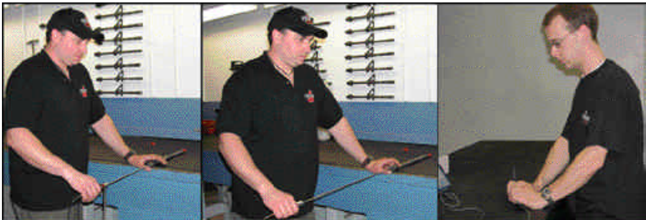
Above: In between each stage of barrel manufacture the barrels are tested using several methods. Left to Right; Air Gauge testing, Bore Scoping and lastly, tested utilizing an Eddy Current.
