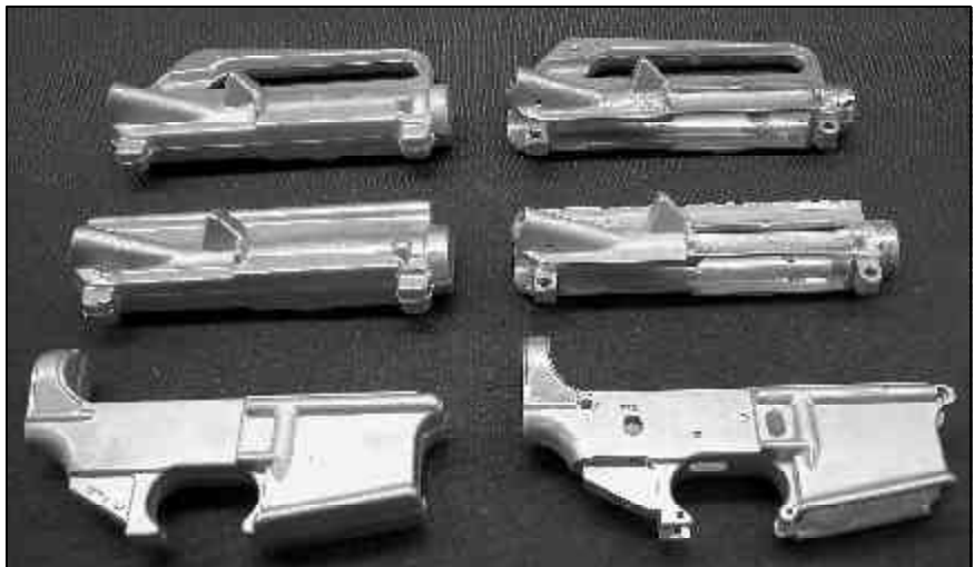
Above & Below: Initial forgings of Bushmaster upper and lower receiver assemblies on the left with their machined counterparts to the right. After machining is done they still must pass another stage of inspection before being finished with a baked dry-lube film and Hard Anodized with a Nickel Acetate final seal coat.
