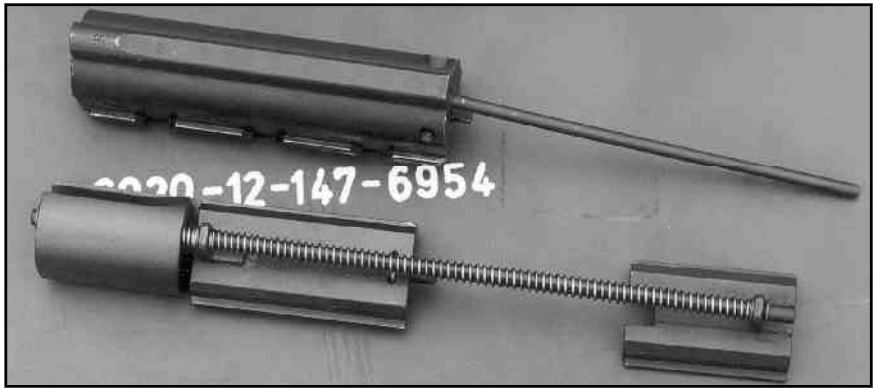
Above: The L12A1 breech block assembly below a standard L1A1 bolt.
