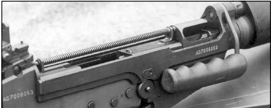
Below: The breech block assembly secures the barrel against the chamber.
