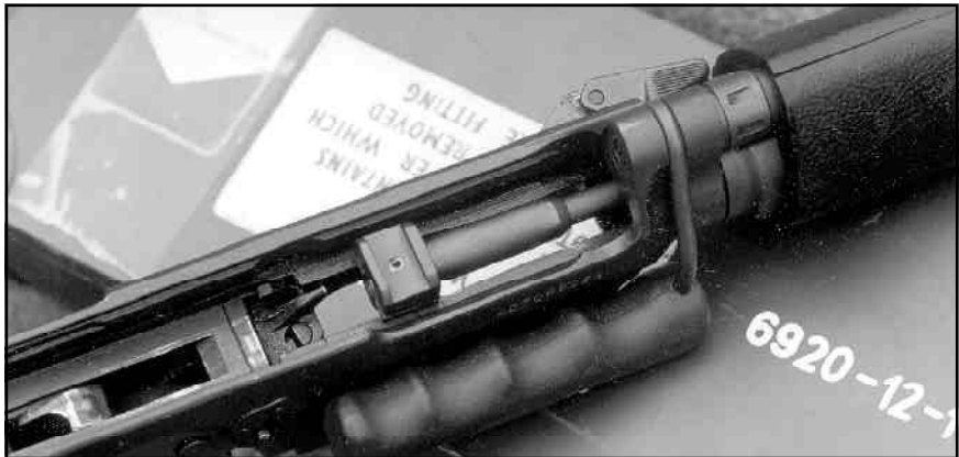
Above: The subcaliber barrel is inserted into the bore from the from the breech end.
