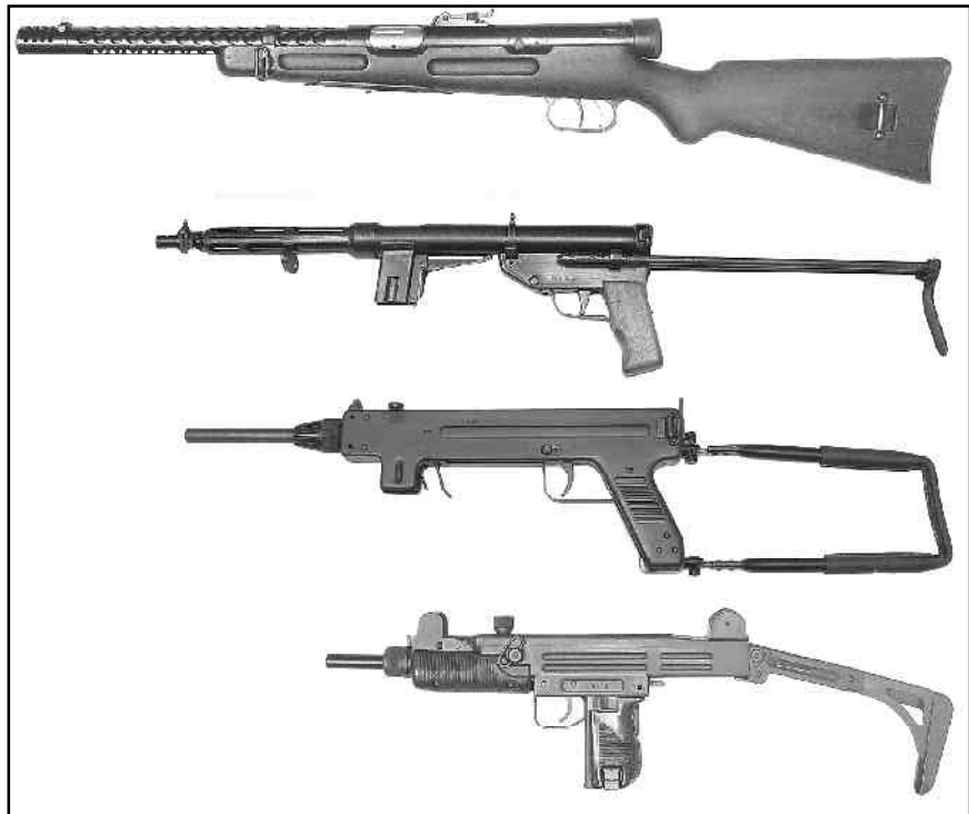
Above: Top to bottom - Beretta M38a, Giandoso TZ-45, Madsen M50 and an Uzi. The Beretta is a first generation Submachine gun. The TZ-45 and the M50 are second generation. Both have grip safeties that are deactivated by the non-shooting hand. The Uzi is a third generation submachine gun. Its grip safety is deactivated by the shooting hand.
