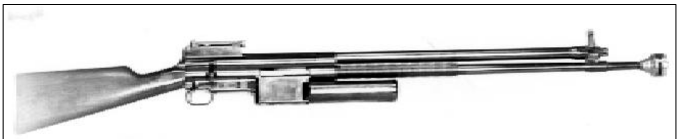
Above: Lewis's second assault rifle modification of his famed original machine gun was a 14-pound weapon using a BAR style magazine. The inventor was still not satisfied and worked to design an even lighter and more effective military weapon. Credit: Savage Arms Company.
